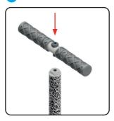
6 Attach connecting hose with I4mm spanner
