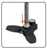
5 Attach connecting hose with 14mm spanner
