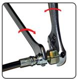
Fully tighten hose connector joint using appropriate spanners.
