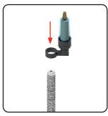
Push down over o-rings to contact with shoulder (rotate to required position)
